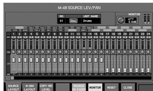
2. Move the cursor to the faders and pan knobs of sources 1–40, and use the value dial to edit the values.
