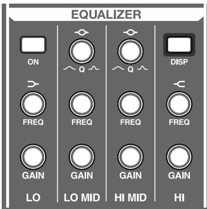
1. Press [ON] to turn the four-band EQ on/off.
