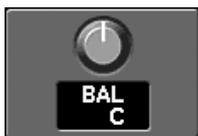
This adjusts the left/right output balance sent from stereo-linked MATRIX channels in the range of L63–R63.
