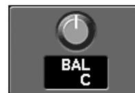
This adjusts the left/right output balance sent from MAIN L/R or stereo-linked AUX channels in the range of L63~R63.
