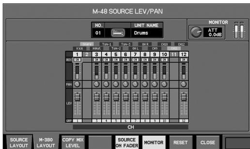
This shows the sources as they are seen from the M-380's fader module section. This display will change according to the M-380's channel layer.
