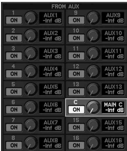
The send from the AUX used by the LCR SYSTEM as MAIN C to the MATRIX is indicated as “C.” This can be used as a send from MAIN C to a MATRIX.
