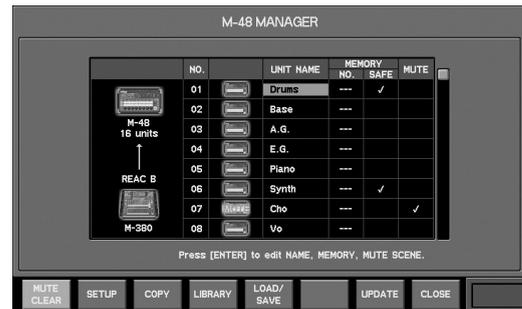
2. In the M-48 list, move the cursor to the UNIT NAME of the desired M-48 and press [ENTER].
