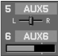
If the AUX send destination is stereo-linked, this lets you adjust the left/right panning of the audio signal in the range of L63–R63. This is shown in the area of the odd-numbered AUX send.
