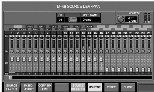
This shows the sources arranged in order of their number (the order in the M-380's REAC B output patchbay).
