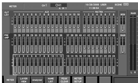
2. Press [F3 (Analyzer)] to access the Analyzer tab.
