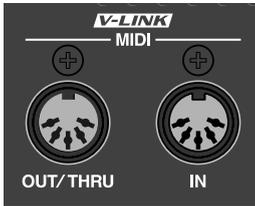
These connectors are for connection with MIDI equipment. An IN connector (for reception) and an OUT/THRU connector (for transmission and “thru”) are provided. You can use the REMOTE popup to switch between the OUT and THRU functions. For details, refer to “Remote settings” (p. 166).
