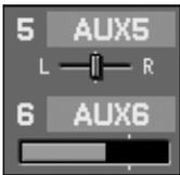
If the send-destination is a stereo-linked pair of AUX channels, this slider adjusts the left/right position in the range of L63~R63. This is shown for the odd-numbered AUX send.
