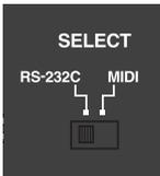
On the M-380 you can use either the MIDI connectors or the RS-232C connector. This switch selects the connector(s) you will use.
