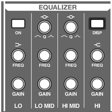
In this area you can operate the four-band EQ that is provided on each channel.
