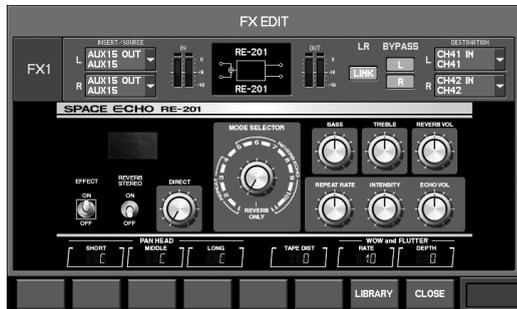
This is a delay that models the Roland RE-201 Space Echo. The original was mono-in, mono-out, but this modeling adds PAN HEAD SHORT/MIDDLE/LONG settings and a REVERB STEREO Sw, allowing you to use it as a mono-in, stereo-out effect. The RE-201 was a very popular product that was produced from 1974 to 1987.
