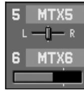
If the send-destination is a stereo-linked pair of MATRIX channels, this slider adjusts the left/right position in the range of L63–R63. This is shown for the odd-numbered MATRIX send.
