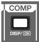
1. Holding down [SHIFT] and pressing [DISP] for the COMP area switches the compressor on or off.
