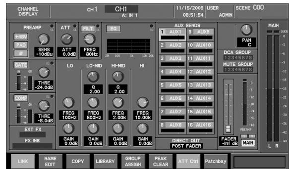
Even if you don't access the CHANNEL DISPLAY screen, the value of the currently-operated parameter is shown in the sub display area when you operate an dial in the CHANNEL EDIT section.
