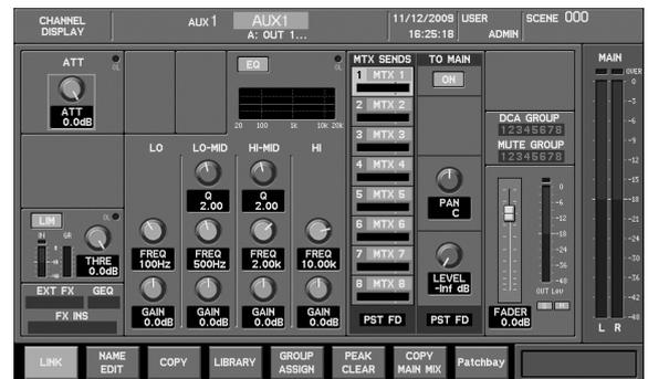
Even if you operate the knobs of the CHANNEL EDIT section without accessing the CHANNEL DISPLAY screen, the value of the currently-operated parameter is shown in the sub-display area.
