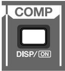
1. Holding down [SHIFT] and pressing [DISP] for the COMP area switches the limiter on or off.
