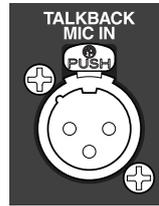
This is a balanced XLR-3-31 female input jack for connecting a talkback mic. Make connections after first checking the wiring diagrams of other equipment you intend to connect.
