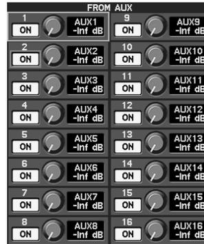
These adjust the send levels from AUX1-AUX16 to MATRIX. The FROM AUX sends are structured as follows.
