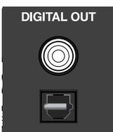
These jacks output a consumer format (IEC-60958 compliant) digital audio signal. Two types of jacks are provided: coaxial and optical. The same digital audio signal is output from both jacks. By default, MONITOR L/R is patched to these jacks.
